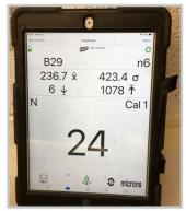
Traceability is maintained with reference to the measuring device and probes serial numbers being stored alongside the measurement data. Graphical reporting also available.
