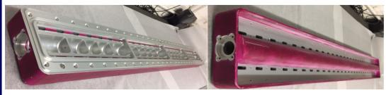
The parts are immersed in Iridite NCP coating for faces which require electrical bonding.
